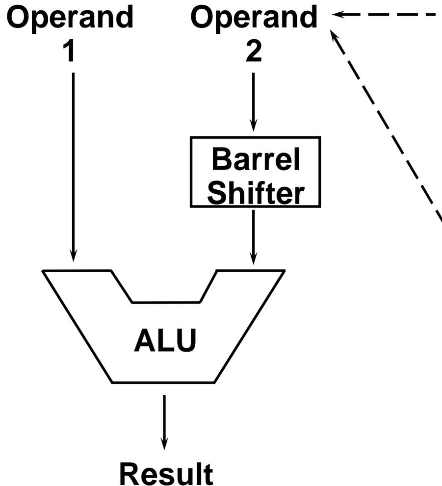
\* **Register, optionally with shift operation applied.**
